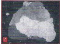
two of the quartz grains are polycrystalline. There are also numerous small angular quartz inclusions <0.1mm in diameter. There are quite a number of small high birefringence grains and a few feldspars are also present.
