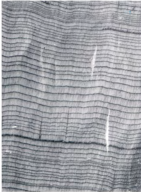
1 Cedrus libani, cross section, 15x, two bands of resin ducts along ring-borders
