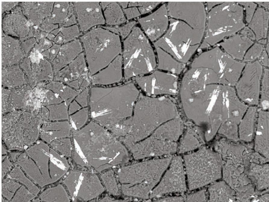
Plate 6 A backscattered electron micrograph of part of the crazed outer glaze surface of the small inscribed fragment from the upper band of inscription. The fragment is shown at the right hand end of the bottom row in Plate 1. The field of view in this micrograph is about 50 micrometres (0.05 mm) wide. The white needle-like crystals in this plate are rich in lead and van.
