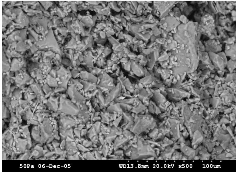
Plate 3. Side view of a fragment showing the microstructure of the body comprising angular quartz fragment ranging from about 60 micrometres down to about 2 micrometres (0.06-0.002mm) in diameter. The field of view is about 250 micrometres (0.25mm) across.
