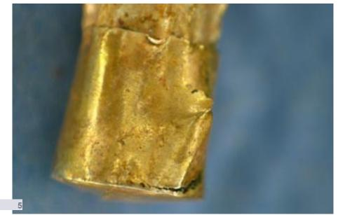
end cap that might correspond to the original join (see the right hand end of fig. 1). Further examination might clarify whether the side joins were soldered.
