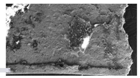
7 A scanning electron micrograph of the inner side of the loose fragment of foil showing the narrow strip of foil (about 0. 03 mm wide) folded under to form a straight edge. The field of view is approximately 0. 5 mm from side to side.
